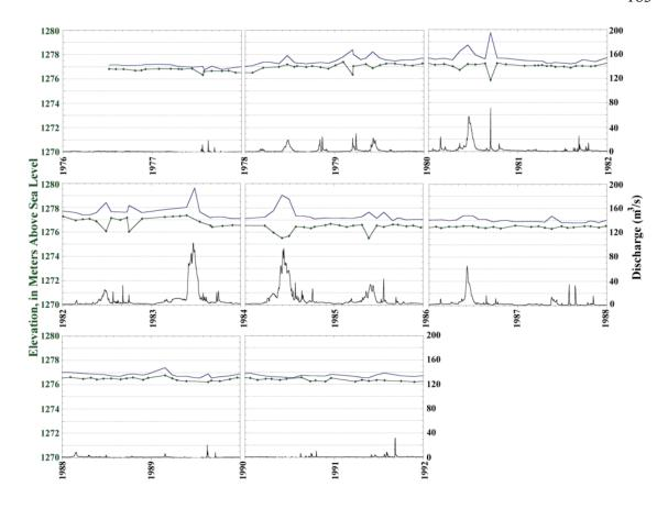
Figure 3.35. Time series of thalweg elevation, water surface elevation and discharge measured from 1976 to 1992. Green data series is the thalweg elevation, the blue data series is the water surface elevation, and the black data series is mean daily discharge.
