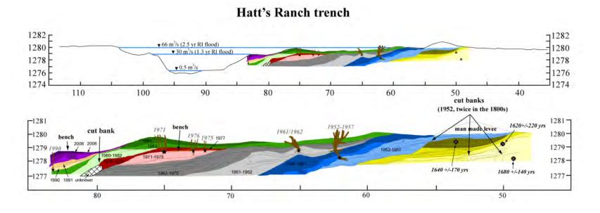
Figure 3.26. Floodplain stratigraphy exposed in trench at Hatt's Ranch. Yellow stars indicate the germination locations of Tamarisk shrubs used in dendrochronologic analyses. Orange and black circles indicates the location where samples were removed for the optically stimulated luminescent analysis. Based on the OSL results, the oldest sediment (shades of yellow and brown packages) was deposited sometime between 1400 and 1840 A.D.
