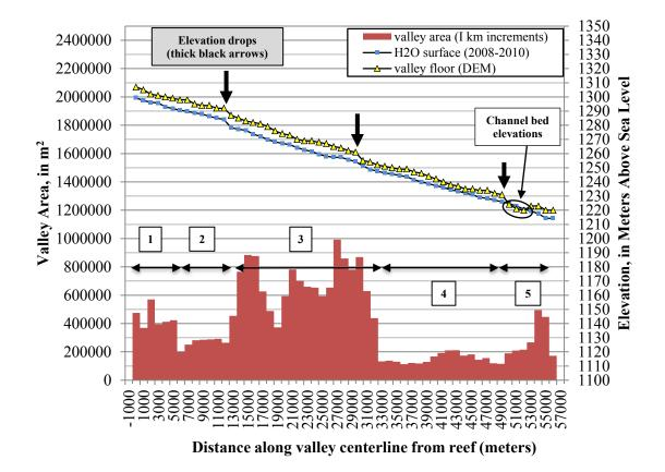
Figure 2.6. Valley area, valley floor elevation, and water surface elevation, plotted at 1-km increments. Elevations were extracted from the 2006 DEM, every 1 km. Aberrant (high or low) data points were adjusted. For a 1-km increment, to convert area (m<sup>2</sup>) to average width (m), divide area by 1000.
