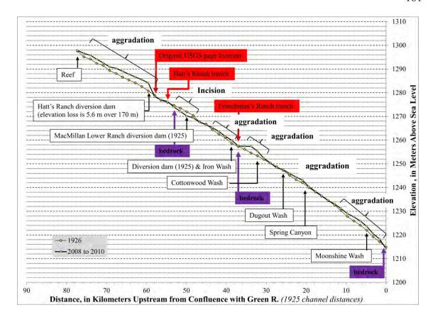
Figure 3.33. Comparison of longitudinal profiles surveyed in 1925 and again in 2008-2010. The long pro comparison shows five segments where aggradation has occurred and one segment where incision has occurred. The 1925 profile was on bedrock in two places and the recent profile is on bedrock in three places.
