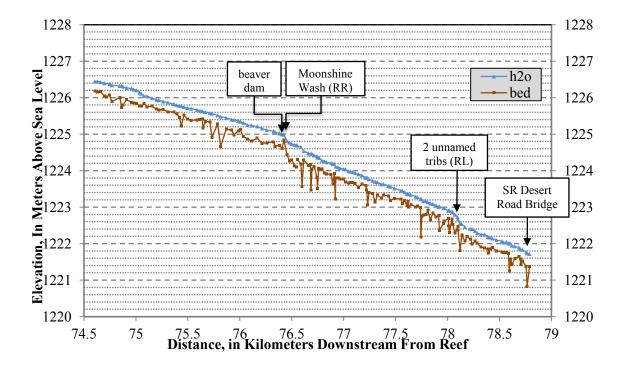
Figure 2.9. Longitudinal profile of a 4-km reach. Reach is located upstream of San Rafael Desert Road bridge. Note the combined hydraulic influence of Moonshine Wash and the beaver dam on the profile, where the slope is gentler upstream of the confluence than it is downstream of the confluence.
