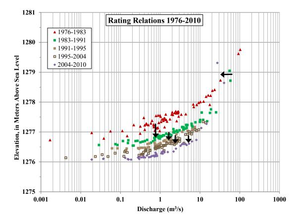
Figure 3.32. Rating relations,1976-2008, measured at the present location of the USGS gage 09328500. Bed elevation decrease is indicated by the downward shift in stage for nearly all discharges. An increase in stage for discharges greater than 30 m³/s for time periods 2004-2010 is caused by reduction in channel capacity, and means that smaller floods are still capable of spilling over the banks and contributing to vertical accretion of the floodplain.
