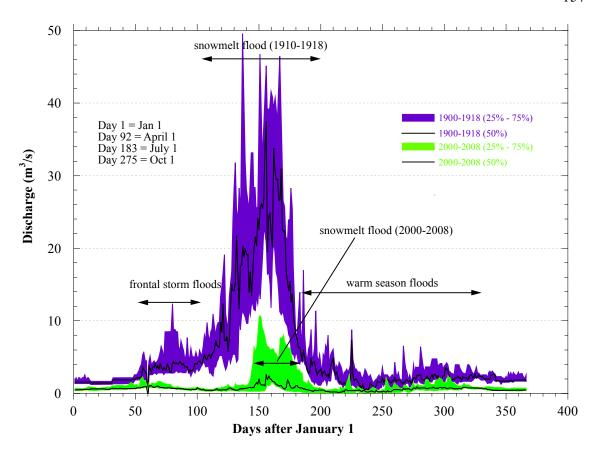
Figure 3.9. Median annual hydrographs for two time periods. The interquartile range for each time period is designated by two colors: purple for 1900-1918 and green for 2000-2008. The black line within each interquartile range is the median stream flow of the time period. There has been a reduction in stream flow between the two time periods for the entire year. The most pronounced reduction in stream flow is evident during the snowmelt flood.
