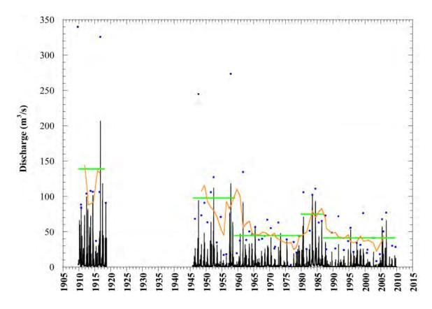
Figure 3.10. Instantaneous annual peak discharge series and mean annual discharge series for the period of record at USGS gage 09328500. Horizontal green lines are the mean annual floods for selected periods. The orange line is a 5-point moving average of the annual peak discharges. Both the moving average and mean annual flood data series indicates a progressive decline in flood peaks over time with the exception of a short period in the 1980s.
