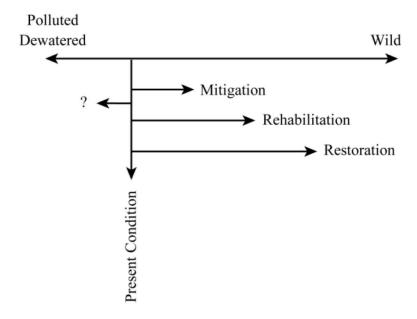
Figure 1.3. Restoration is the return of an ecosystem to its pre-disturbance condition. Rehabilitation is the reestablishment of some attributes of the ecosystem to their pre-disturbance condition. In the case of the San Rafael River, complete restoration is impossible, and policy choices must be made to identify which attributes should be partly restored.
