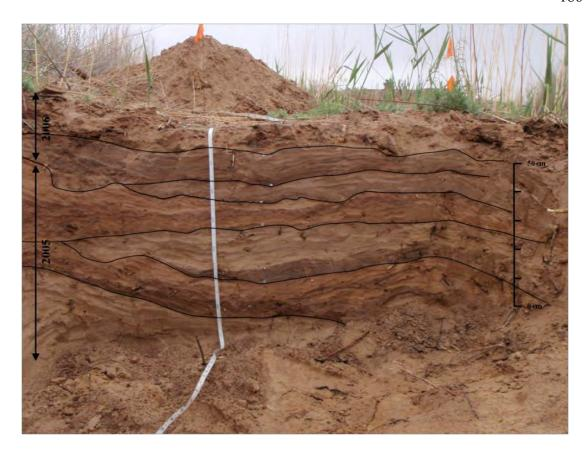
Figure 3.38. Sedimentology of near channel bench exposed in left bank trench at Frenchmans's Ranch trench. The channel is off the right side of the photo.
