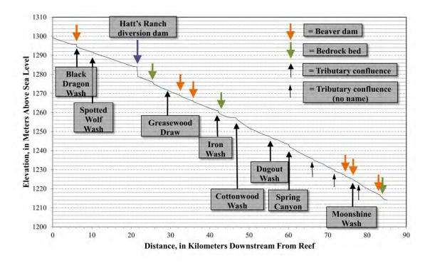
Figure 2.10. Water surface elevation profile in the study area. Data was collected between 2008 and 2010, and has been post processed using orthometric elevations.
