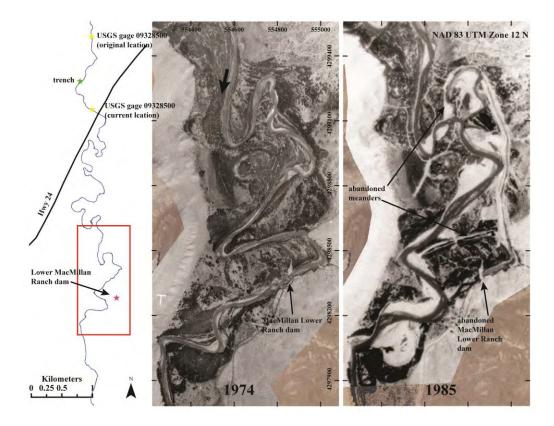
Figure 3.5. Map showing the location of the MacMillan Lower Ranch dam. The 1983 snowmelt flood caused an avulsion which abandoned the meander where the MacMillan Lower Ranch dam was located (identified in both aerial photographs). Another avulsion occurred a short distance upstream, either during the 1983 or 1984 snowmelt flood
