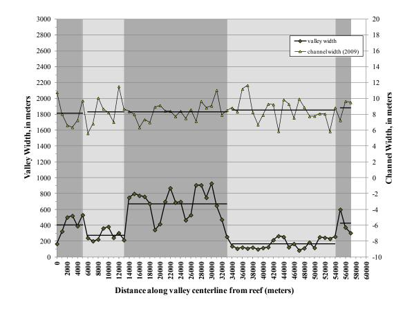
Figure 2.11. Channel width and valley width measured at 1-km valley increments. Also shown is the average channel width and valley width (horizontal lines) for each of the five valley segments in the study area. The average width for each valley segment is the mean of the width values at all 1-km nodes with a segment. Valley segments are denoted by alternating shades of grey.
