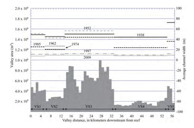
Figure 3.31. Segment average channel width determined from aerial photographs. The average width of the active channel in segment 2 did not change between 1974 and 1985 despite the large snowmelt floods in 1983 and 1984.
