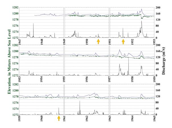
Figure 3.34. Time series of thalweg elevation, water surface elevation and discharge measured at abandoned cableway from 1947 to 1965. The green data series is the thalweg elevation, the blue data series is the water surface elevation, and the black data series is the mean daily discharge. Orange arrows indicate flash floods where bed elevation changes could be determined because of the availability of discharge measurements.
