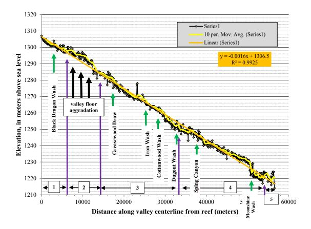
Figure 2.5. Longitudinal profile of the valley in the study area. The elevation data used to create this plot was extracted from an auto-correlated 5 m DEM every 50 to 100 m along the valley centerline. The 5-m DEM was produced from 2006 NAIP imagery and has a 4-m elevation uncertainty.
