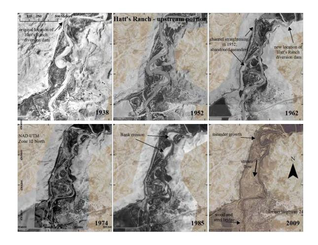
Figure 3.6. Aerial photograph comparison of the upstream portion of Hatt's Ranch. The Hatt's moved the diversion dam to it's current location and straightened the channel in two places in during the winter of 1952/1953, after the aerial photographs were taken in November 1952.
