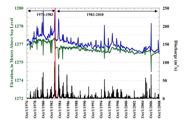
Figure 3.30. Thalweg elevation time series for the time period from 1976 to 2010. The drop in local base level at the downstream location, when the 1983 snowmelt flood bypassed the Lower Macmillan Ranch Dam, is indicated by the red bar. A period of incision from 1983 to 2010 followed the downstream drop in base elevation that occurred during the 1983 snowmelt flood. There is no apparent trend in bed elevation change between 1976 and 1983.
