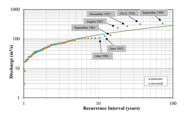
Figure 3.48. Flood frequency at USGS gage 09328500. We calculated the flood frequency shown here using the instantaneous peak annual flood series. Monsoon floods are those that occur between July 1 and December 31. Snowmelt floods occur in April, May, and June.
