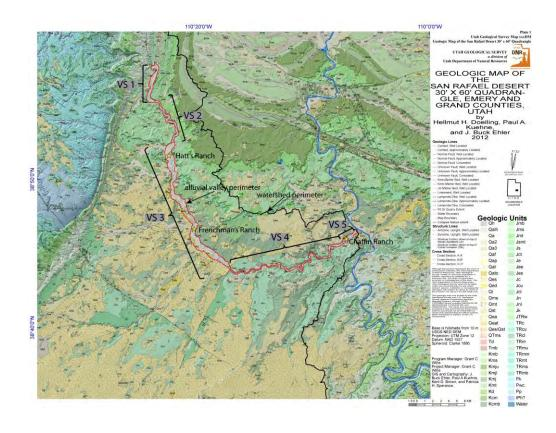
Figure 2.7. Geology of the study area. The map is modified from Doelling et al. (2014). The perimeter of the alluvial valley of the study area is indicated by a red line. The perimeter of the San Rafael River watershed is indicated by a black line. Important places in the study area are indicated by yellow stars. The correlation of map units that are encountered along the study area at valley elevation is shown in Figure 2.8.
