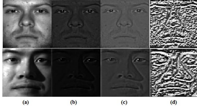
Fig. 4.2: Illustration of the intermediate results obtained by the three steps of the proposed AH-ELDP method. (a) Original face images; (b) Homomorphic filtered images; (c) Enhanced filtered images; and (d) AH-ELDP images after extracting eight local directional patterns.
