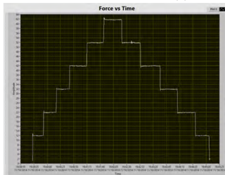
(d) Loading and Unloading Diagram during Calibration
