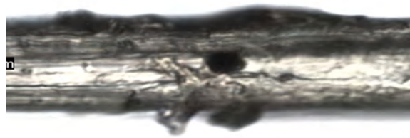
(a) Fiber Delamination
