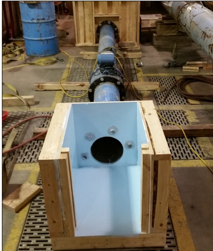
Figure 6. Third box built with a sluice gate.
