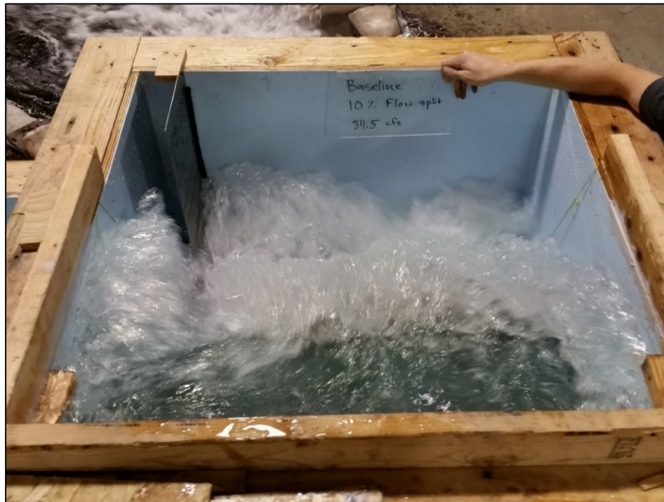
Figure 11. Config. 1-Baseline with the high flow of 8 cfs.
