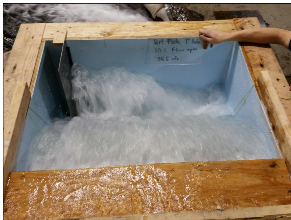
Figure 12. Config. 1-6 with the high flow of 8 cfs.
