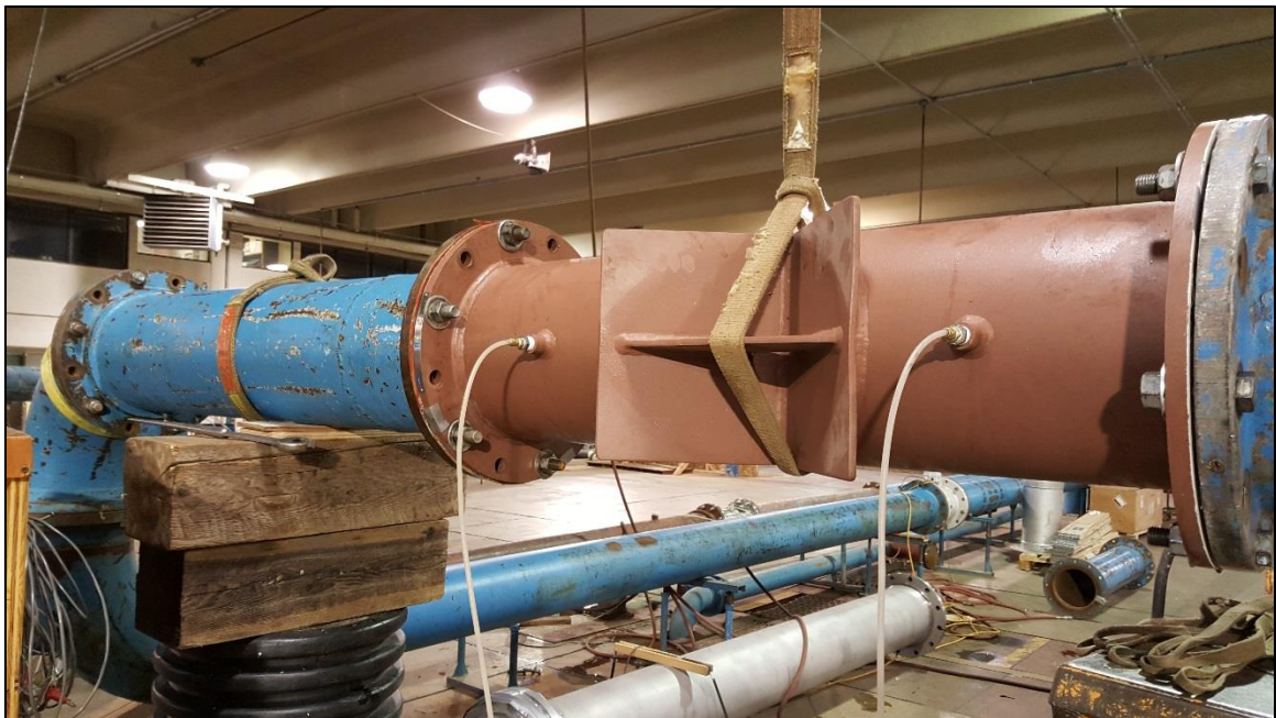
Figure 6: Horizontal or Out-of-Plane Installation of Wedge Flowmeter
