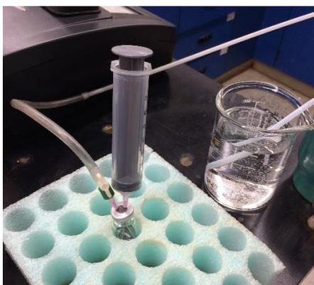
**Figure 6.** Setup for creating the helium headspace in vials used to measure  $^{15}\text{N}_2$ . Helium is constantly bled into the vial through the tubing on the left while water is pulled from the vial using the syringe on the right. Helium is also allowed to flow out of the tubing inserted in the beaker of water so that the vial does not become pressurized during creation of the helium headspace.
