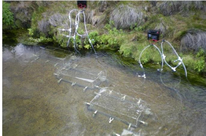
**Figure 5.** Installed chambers in the field. Pumps and batteries are arranged on the bank in order to keep the batteries dry and allow easy access to the sampling ports.
