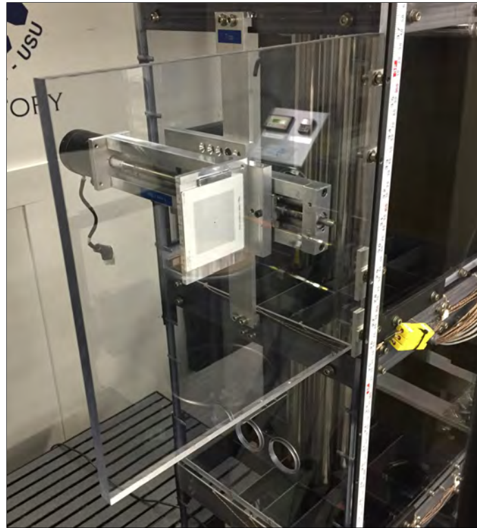
Fig. 3.15: Calibration setup used for acquiring the SRQ velocity data.
