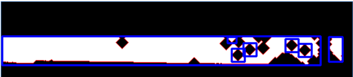
Figure 3.11 Bounding Rectangles drawn for all contours in image with white landing pad
