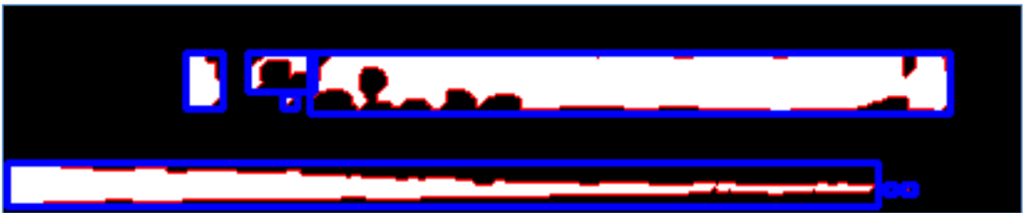
Figure 3.10 Bounding Rectangles drawn for all contours in image with green landing pad
