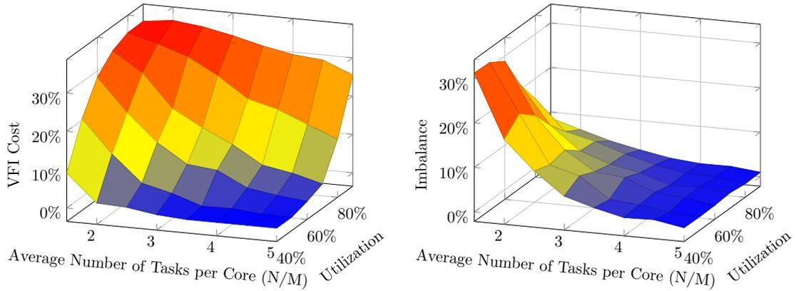
Fig. 6.2: Combined average VFI cost (left) and imbalance (right) (i.e., combined average of two, four, and eight cores per VFI), as a function of the average number of tasks per core (i.e.,  $N/M$ ) and system utilization.
