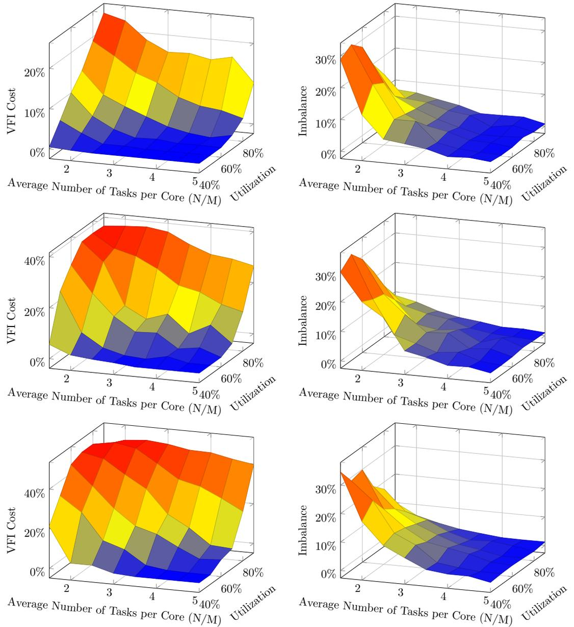
Fig. 6.1: Average VFI cost (left) and imbalance (right) for two (top), four (middle), and eight (bottom) cores, as a function of the average number of tasks per core (i.e.,  $N/M$ ) and system utilization.
