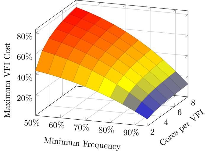
Fig. 4.1: The maximum VFI cost (Equation 4.7) as a function of the number of cores ( $M$ ) by the minimum frequency ( $f_1$ ) that the VFI can reduce to (as a percentage of the maximum frequency,  $f_K$ ) assuming a pure CMOS circuit (i.e.,  $w_k \propto f_k^3$ ).
