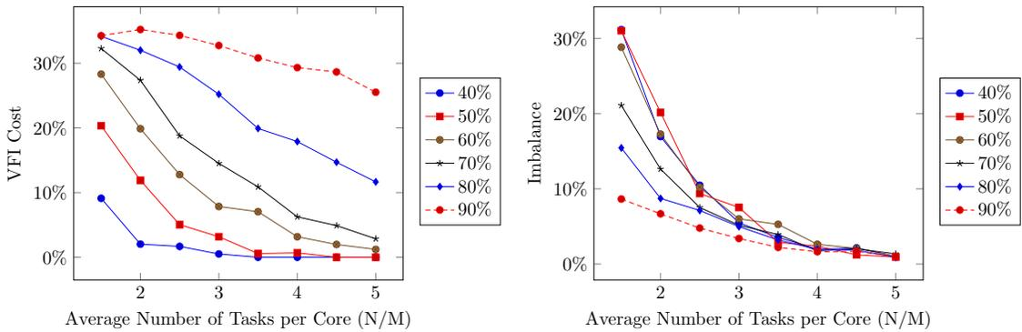
Fig. 6.4: Combined average VFI cost (left) and imbalance (right) for the system utilization by the average number of tasks per core ( $N/M$ ).
