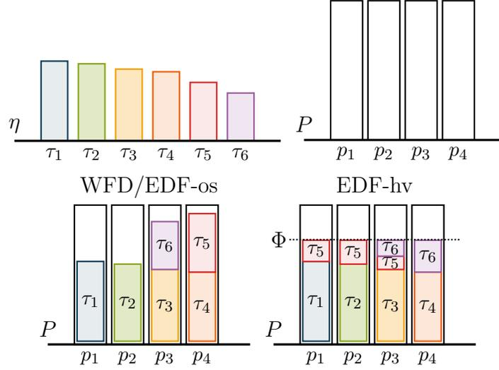
Fig. 5.1: Partitioning the task set,  $\eta$  (top left), where each task is represented by its utilization, onto the set of cores,  $P$  (top right), using the WFD (or EDF-os; bottom left) and EDF-hv (bottom right). EDF-hv restricts the available capacity of each core to  $\Phi$ .
