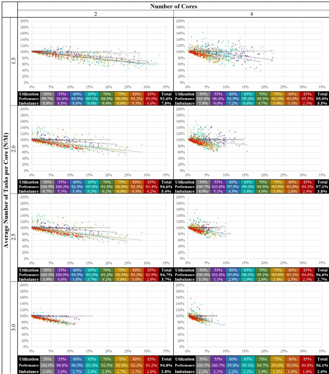
Fig. 6.5: Reduction in energy consumption (i.e. performance) of EDF-hv compared to WFD versus the imbalance of WFD for two- and four-core systems with one VFI and task sets with 1.5, 2.0, 2.5 and 3.0 average number of tasks per core (i.e., N/M).
