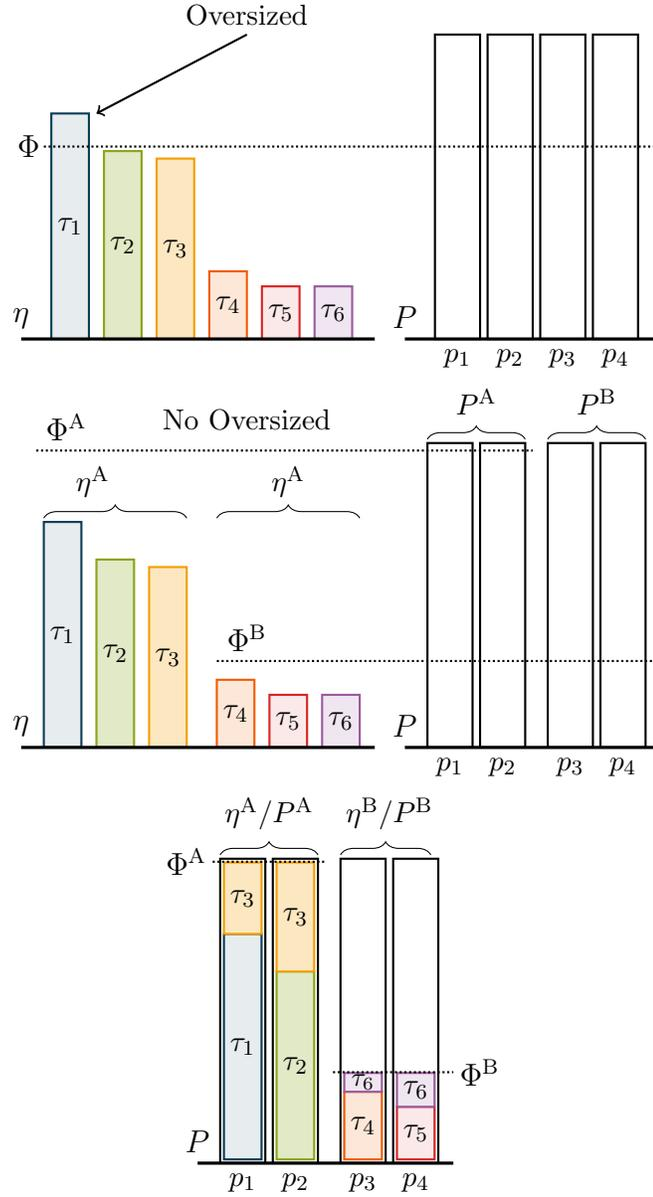
Fig. A.2: An example of horizontal multi-partitioning (HMP). The original task set,  $\eta$  (top; where each task's utilization is shown), has one oversized task,  $\tau_1$ . As such,  $\eta$  is divided into two subsets,  $\eta^A$  and  $\eta^B$ , as well as  $P$  is also divided into two subsets,  $P^A$  and  $P^B$  (middle). Although the resulting subsets no longer have any oversized task, the system is clearly not load-balanced (bottom).
