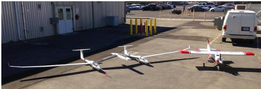
**Figure 2. Demonstration Prototype of Towed-Air Launch Platform**
