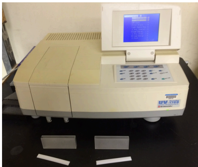
Figure 16. Shimadzu UV-1700 PharmaSpec UV-Visible Spectrophotometer instrument with 10 cm path-length cells.
