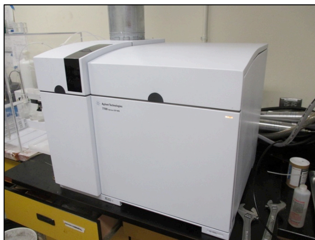
Figure 14. Agilent 7700x ICP-MS.
