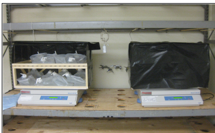
Figure 10. ThermoScientific MaxQ 430 HP Orbital Shaker tables. Left - Uncovered with cubitainers. Right - Covered to exclude ambient light.
