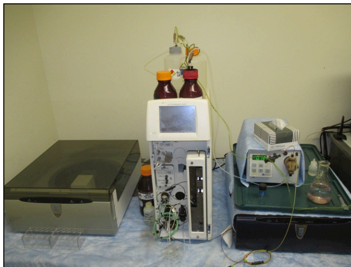
Figure 15. Dionex ICS-1600 Ion Chromatography instrument.
