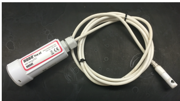
Figure 6. HOBO Pro v2 external temperature/relative humidity data logger.
