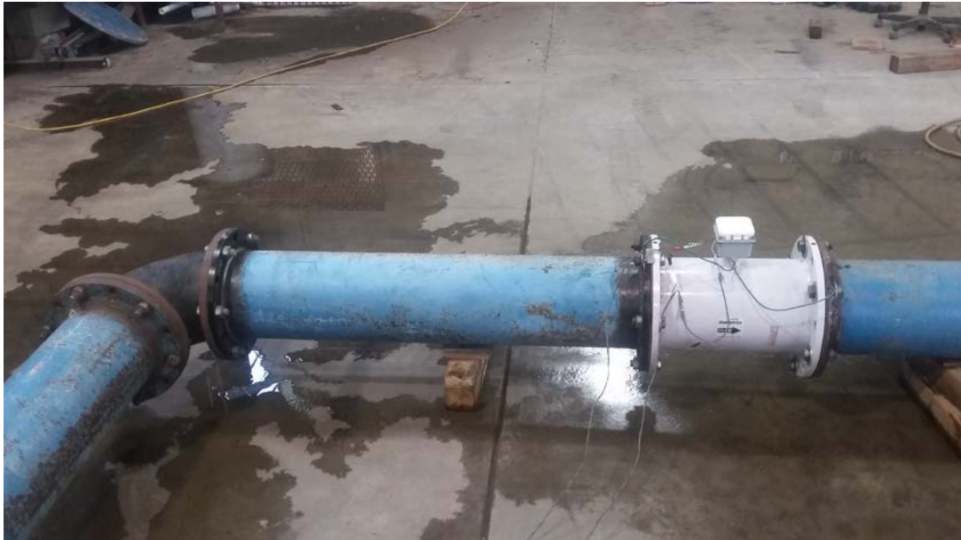
Figure 9. Phase II Elbow Setup for 5D Test (flow left to right)
