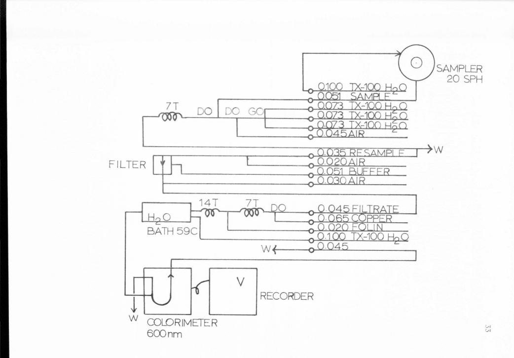
to be improved if an air bubble was inserted just after uptake of the non-casein protein filtrate. The non-casein protein filtrate was first mixed with the copper solution (reagent C) and then with the Folin-Ciocalteau phenol reagent. After thorough mixing in 14 turns of coiled glass tubing, the reaction system was passed through a 59C waterbath for 3 minutes. The blue-violet color was read at 600 nm in the colorimeter and recorded continuously on the recorder module.
