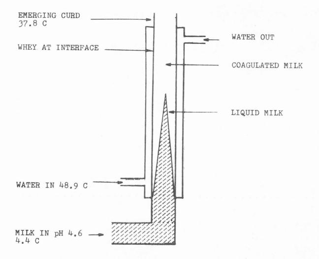
that it had a provision for periodically reversing the flow of coagulating milk to prevent sticking in the coagulation tubes.
