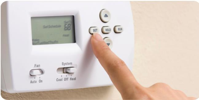
Space heating is the chief consumer of energy in the home - followed by water heating. Programmable thermostats can help reduce this energy drain.
