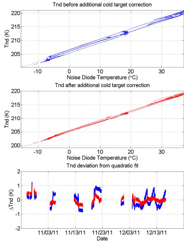
**Figure 4: Top: Noise Diode Excess Temperature as a function of Noise Diode Temperature. Middle: Noise diode excess temperature after the additional cold target correction. Bottom: Noise diode excess temperature deviation from quadratic fit**
