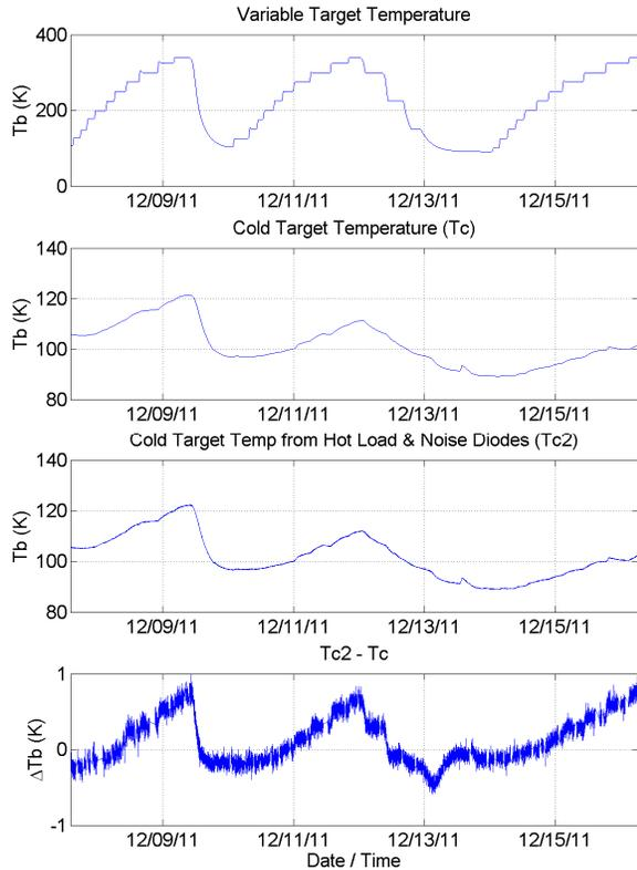
**Figure 3: Top: Variable target temperature over the duration of the GMI calibration test. 2<sup>nd</sup> from Top: Cold target-measured brightness temperature using PRTs in the target. 3<sup>rd</sup> from Top: GMI-measured cold target brightness temperature (36 GHz) using the hot load and noise diodes as calibration references Bottom: Difference between cold target temperature and the GMI-measured cold target brightness temperature**
