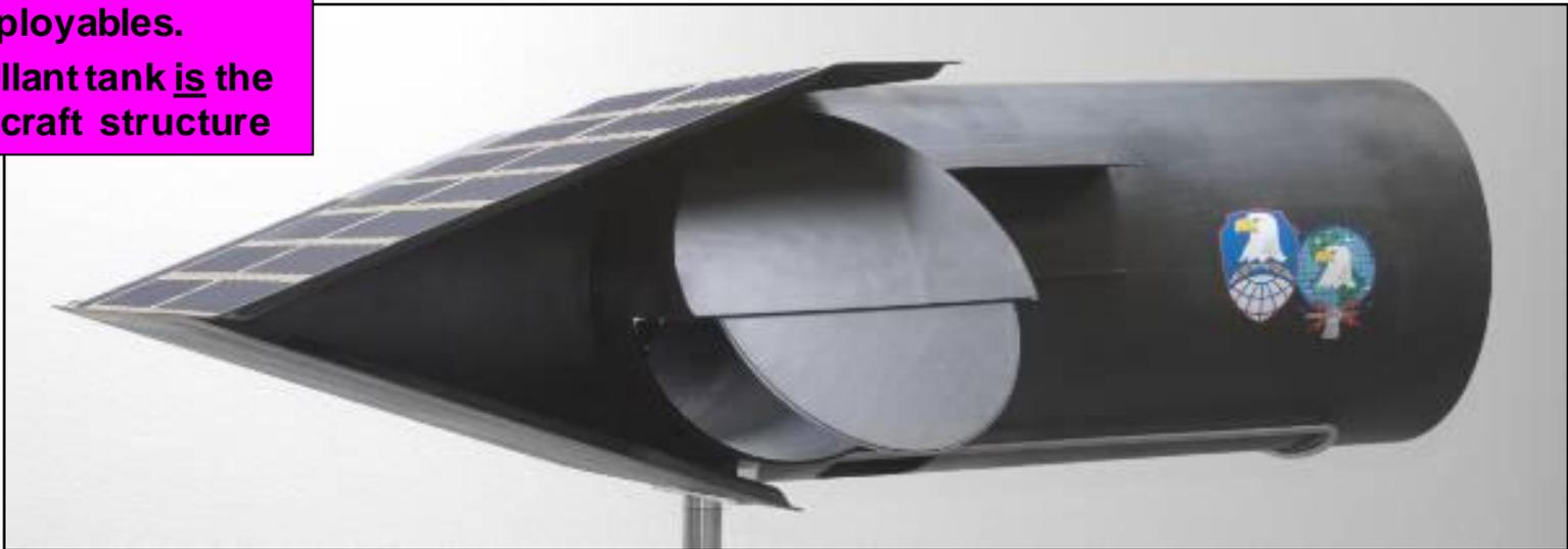
**Spacecraft configuration designed to minimize drag and torque with large propellant volume.**
