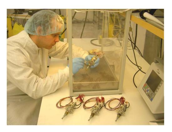
Assembly of Flight Thrusters
