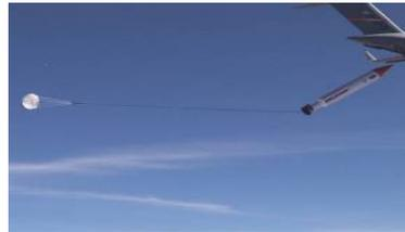
C-17 drop test of simulated QuickReach™ Small Launch Vehicle
