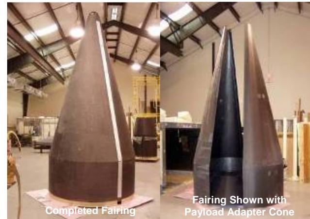
Completed Fairing      Fairing Shown with Payload Adapter Cone
