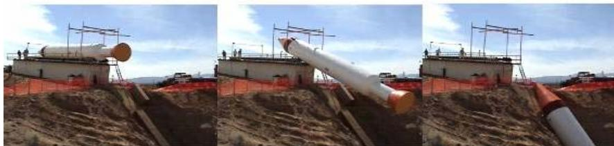
Full-scale ground drop tests
