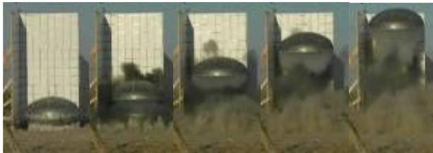
Stage separation test of full-scale diameter test article
