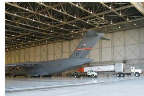
QuickReach™ drop test article loaded into C-17 aircraft
