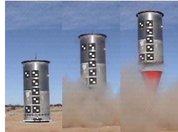
Full-scale stage separation test
