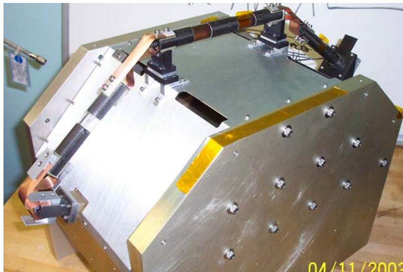
Boom Stowed in structural mockup vibration fixture
