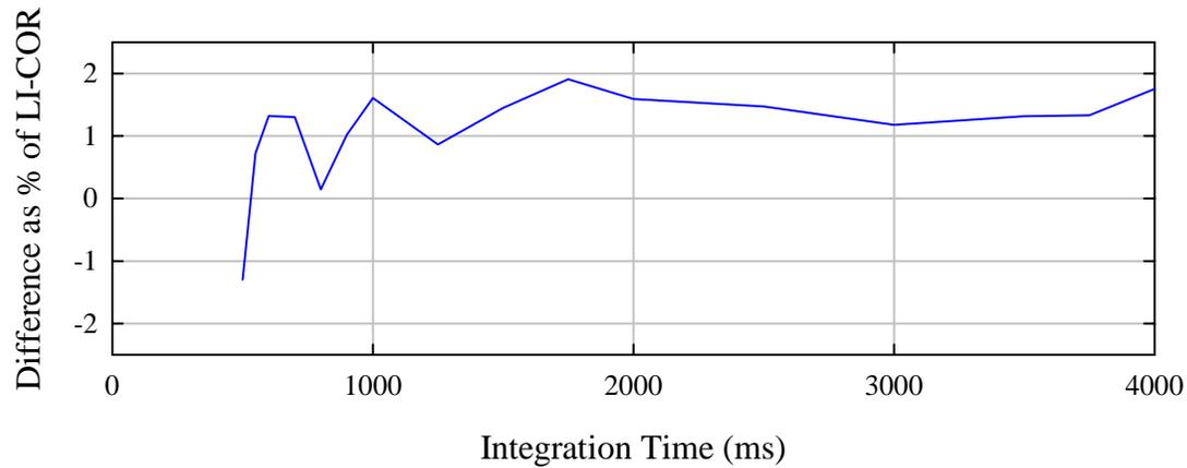
**FIGURE 2** The effect of changing integration time from 500 ms to 4000 ms. Measurements were made under an incandescent lamp. The calibration time was 100 ms. The radiation varied from 30 to 300  $\mu\text{mol per m}^2 \text{ per s}$ . Changes were less than 2% in all cases.
