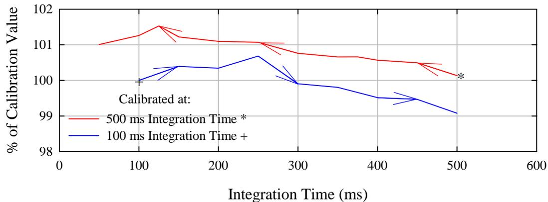
**FIGURE 1** Effect of changing integration time on measurement accuracy. The red line shows the effect of **decreasing** integration time. The blue line shows the effect of **increasing** integration time. Changes are less than 1.5% in both cases.
