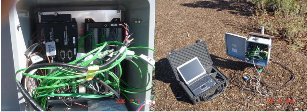
Figure 6 Data was collected with two CR1000 data loggers and AM 16/32 Multiplexers and stored on CFM 100 Compact Flash Memory modules with 1 GB Flash memory drive (Campbell Scientific, Logan, UT).
