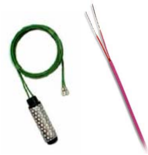
Figure 5 Inexpensive Irrrometer Watermark™ 200 resistance block (Riverside, Ca.) left and Omega Engineering Type E Thermocouple, right. Watermark blocks measured electrical resistance from a 250 mV electrical pulse between double coiled wires imbedded in the granular matrix material.
