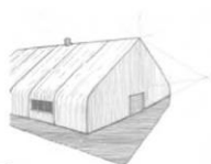
80' - 90' WIDE SPRUNG STRUCTURE 22,000 FT 2 FIRM STRUCTURE
