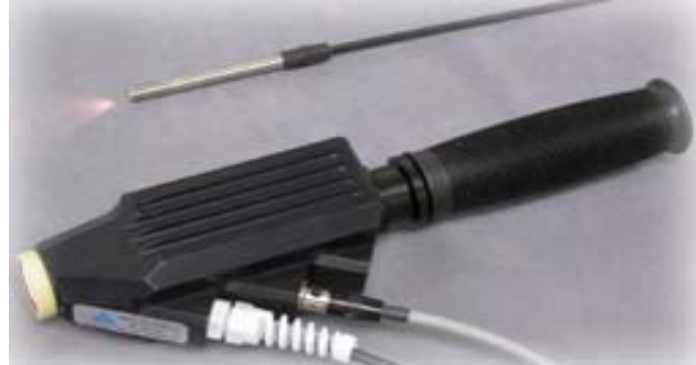
Figure 10: StellarNet (top) and ASD reflectance probes.
