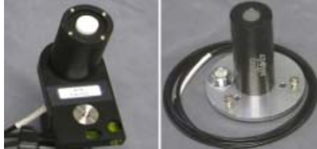
Figure 11: ASD (l) and Apogee/StellarNet cosine diffusers.
