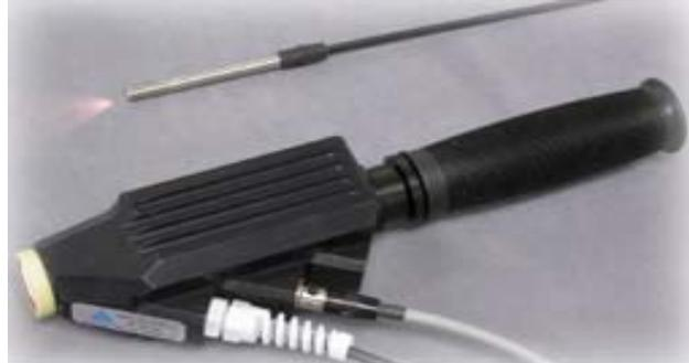
**Figure 10: StellarNet (top) and ASD reflectance probes.**
