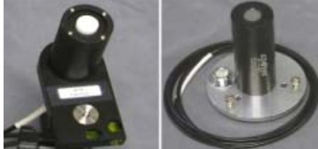
**Figure 11: ASD (l) and Apogee/StellarNet cosine diffusers.**
