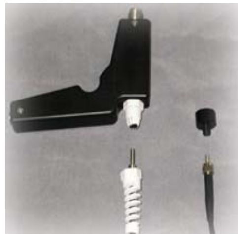
Figure 9: Cable connectors for ASD pistol grip and Apogee/StellarNet cosine head.
