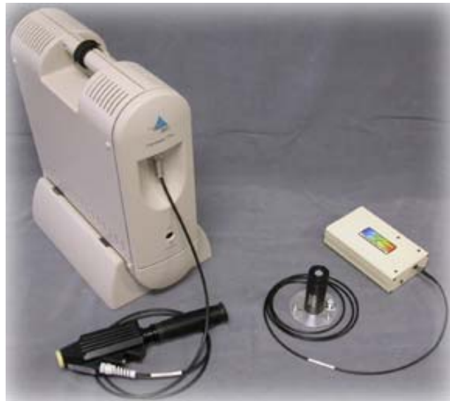
Figure 1: (l-r) ASD FieldSpec Pro JR, Apogee/StellarNet SPEC-PAR/NIR, and StellarNet dual InGaAs-Vis/NIR
