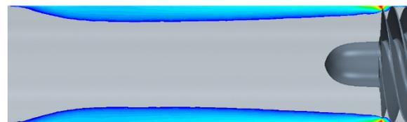
Figure 1 Reversed flow from the blade tip can create instabilities in the flow
