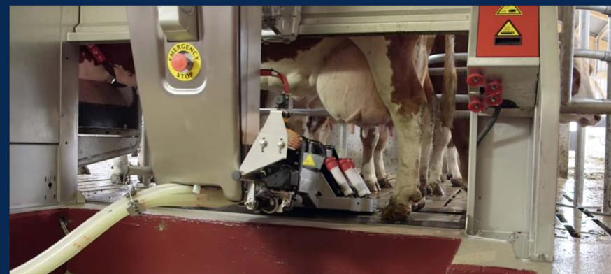
View from the backside— “screen side”—of the LELY Astronaut, an AMS, showing the arm going underneath the cow, preparing to attach the cups post cleaning.
