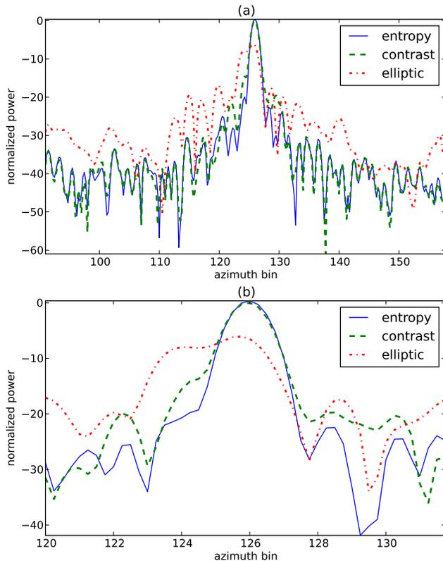
Figure 4. Azimuth slices through one of the autofocused point targets from Fig. 3 for each autofocus cost function. The lower plot (b) shows a zoomed-in region around the central peak.
