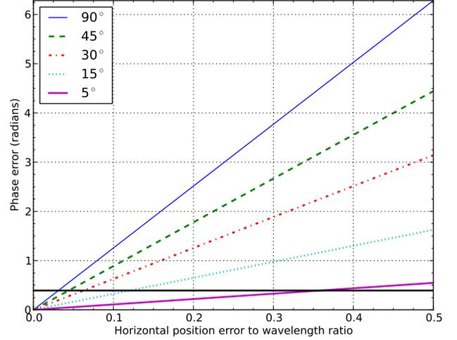
Figure 1. Estimate of the phase error for position estimate errors as a function of the ratio of position error magnitude to wavelength. Multiple lines are shown for various coordinate to slant-range ratios. The horizontal line marks the phase  $\pi/8$ .
