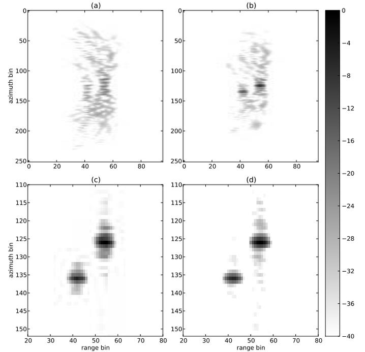
Figure 3. Backprojected images in dB of simulated data with two point targets. (a) shows the original image and (b-d) show autofocused results for various cost functions: (b) elliptic, (c) maximum contrast, and (d) minimum entropy.
