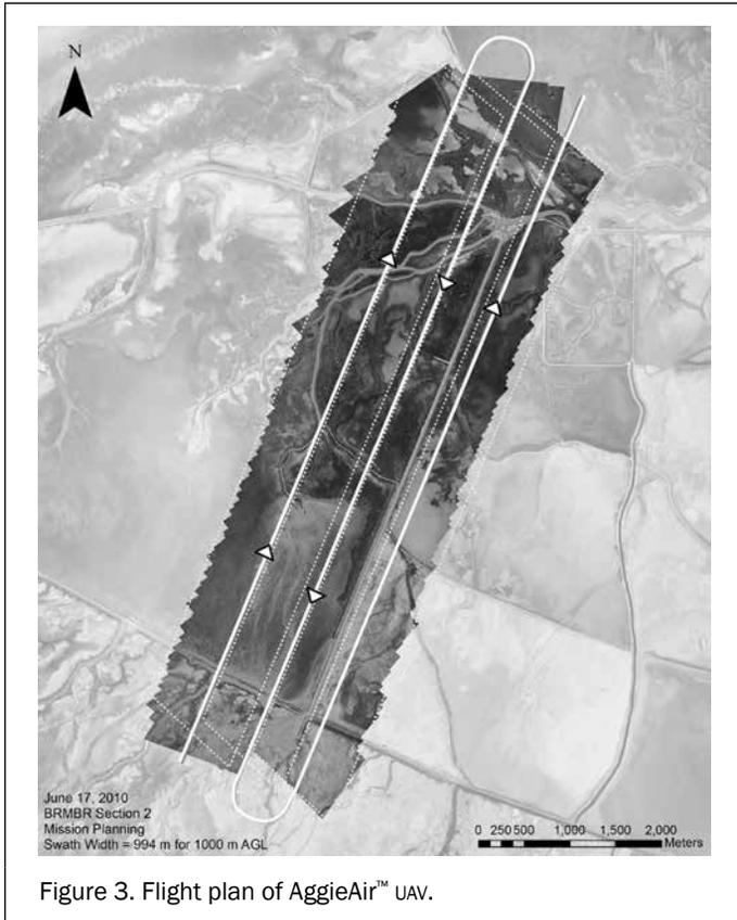
Figure 3. Flight plan of AggieAir™ UAV.
