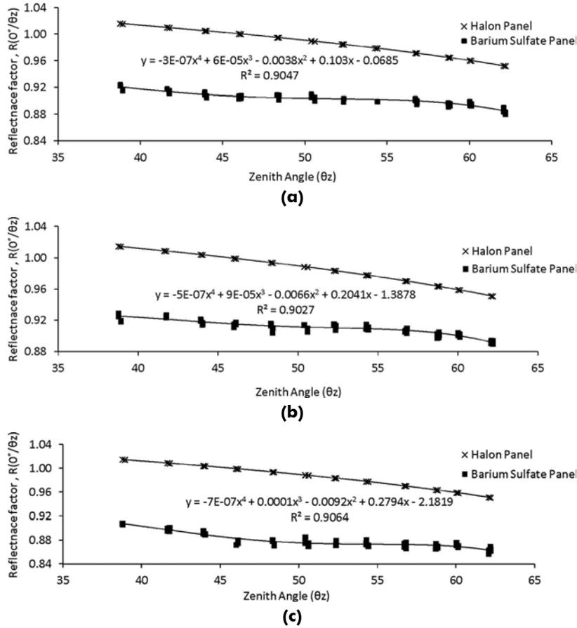
Figure 8. Panel cross calibration results showing coefficients of BaSO<sub>4</sub> panel: (a) Reflectance factor as a function of solar zenith angle for red band, (b) Reflectance factor as a function of solar zenith angle for Green band, and (c) Reflectance factor as a function of solar zenith angle for NIR band.
