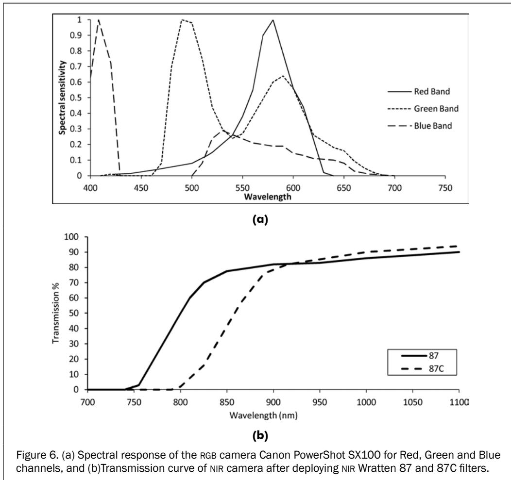
Figure 6. (a) Spectral response of the RGB camera Canon PowerShot SX100 for Red, Green and Blue channels, and (b) Transmission curve of NIR camera after deploying NIR Wratten 87 and 87C filters.
