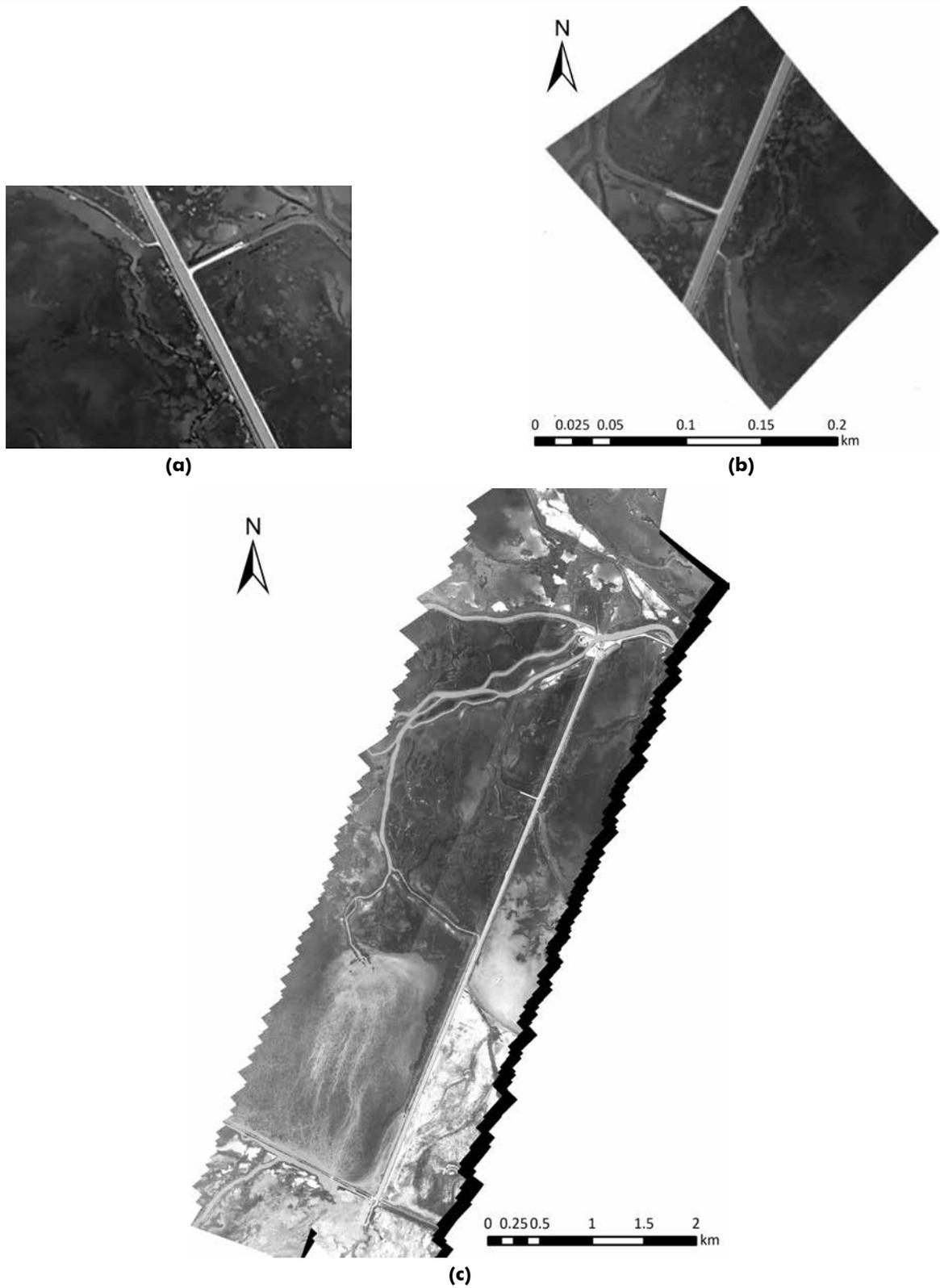
Figure 7. (a) Raw tile from UAV image acquisition, (b) Orthorectified tile, and (c) Orthorectified and mosaicked image.
