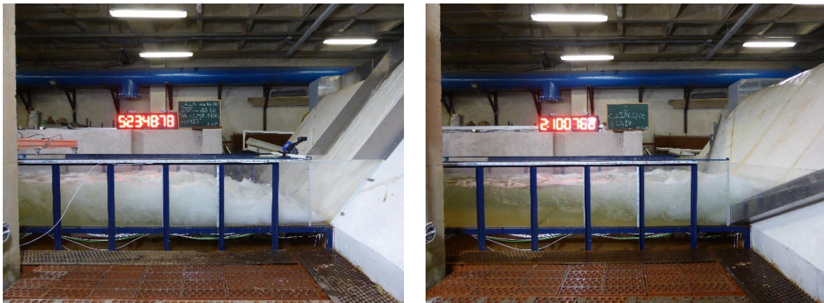
Figure 3. Side view of the performance of the stilling basin for an inlet discharge of 100 ls-1. Left: Hydraulic jump (tailwater depth 0.423 m) with frontal inlet flow. Right: Impingement of HCC jets with frontal flow (tailwater depth 0.417 m).
