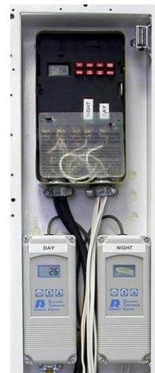
Electronic temperature controllers are connected only to the heating elements in the chamber, while the water flow through the coil remains at a fixed rate (the minimum amount of water required to provide cooling during the day with the lights on).
