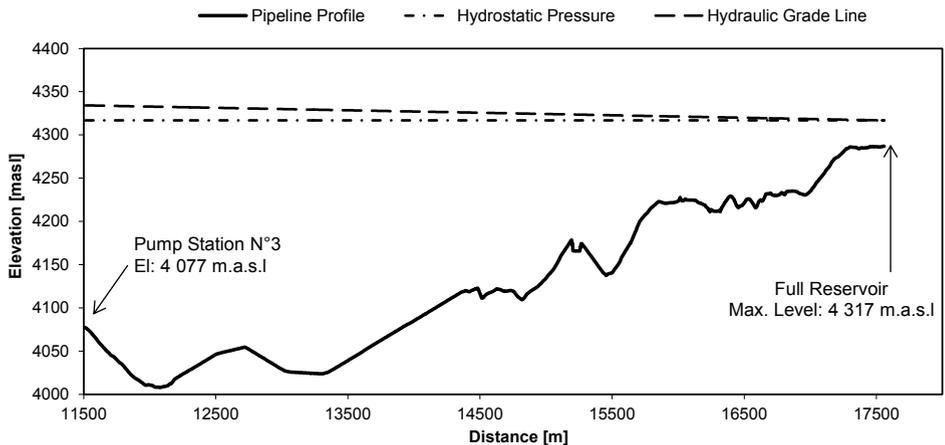
Figure 2 – Hydraulic Grade Line for water pipeline system starting at Pump Station N°3 to the Reservoir. Full-reservoir case.
