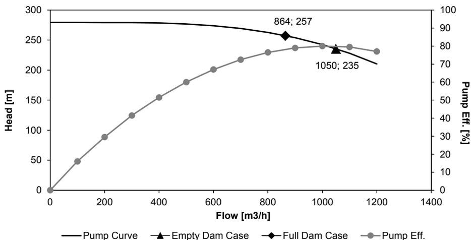
Figure 3 – Operation Points for each pump of the Pumping Station N°3.
