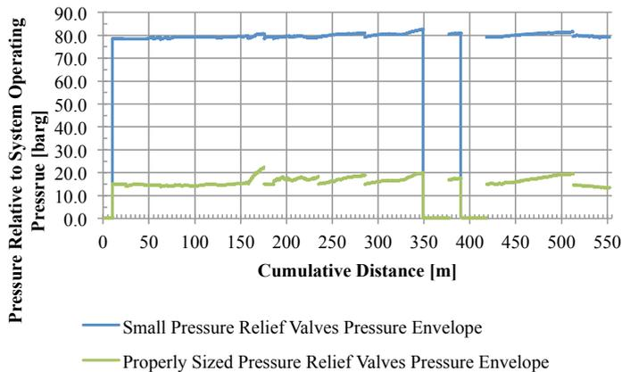
Figure 4 – Isolated Conditions Maximum Pressure-Envelope
