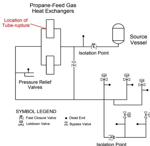
Figure 1 – System Schematic Drawing
