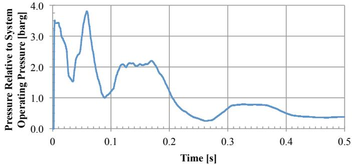
Figure 2 – Tube-rupture Pressure Time-history
