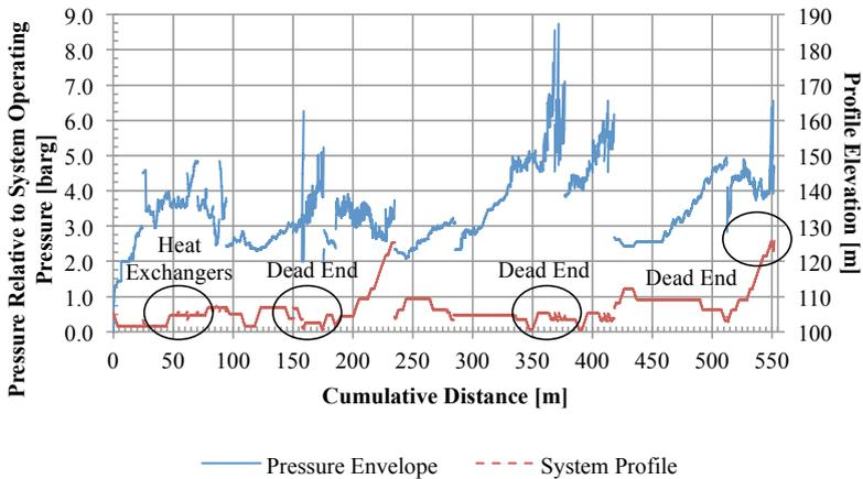
Figure 3 – Normal Operating Conditions Maximum Pressure-Envelope
