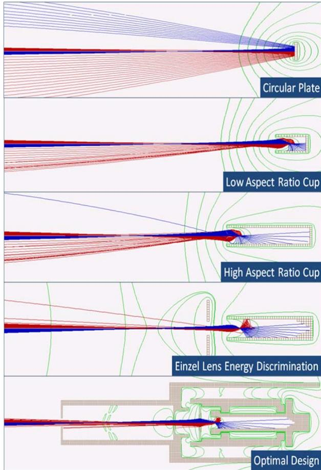
**Fig. 1** - Cross-sectional views of design progression with two consistent incident electron beams to determine energy resolution. The red beam energy is 99.9 eV and the blue is 100.1 eV, with 0.1% resolution. Each design is set to detect only electrons with energies greater than or equal to 100 eV. The green contour curves represent the electric field potentials.
