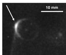
Figure 4. Arrow indicates arc position on sample.
