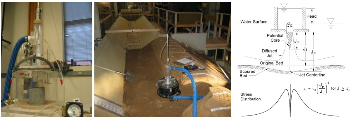
Figure 1: Submerged jet erosion test device for laboratory and in situ use, and a schematic diagram with the stress profile applied to the soil boundary (Hanson and Cook 2004).
