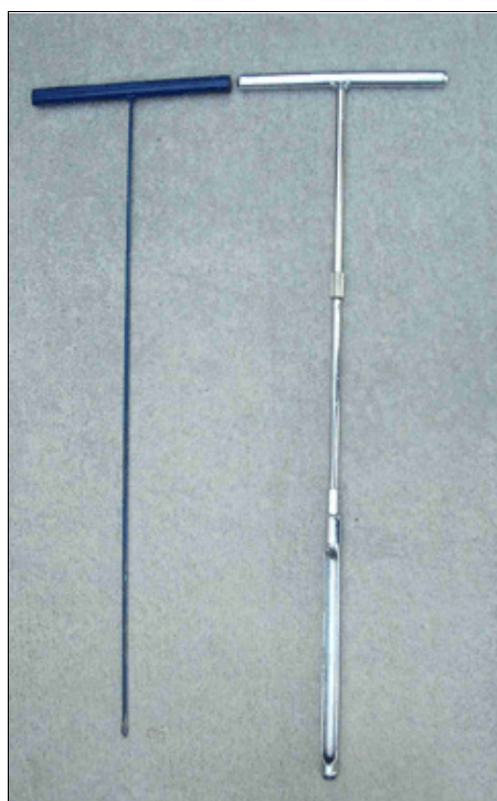
A tile probe (left) and soil probe (right)
