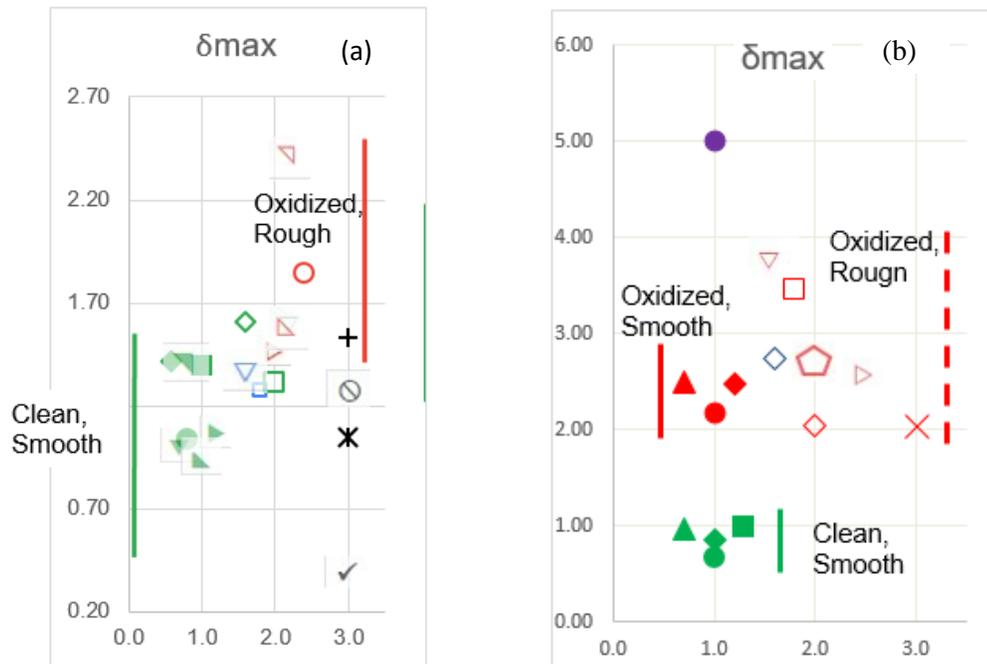
FIG. 4.1.  $\delta_{max}$  values for two conducting materials. (a) Copper and (b) aluminum, included with aluminum is a measurement of  $\text{Al}_2\text{O}_3$  (sapphire) to illustrate an extreme case of oxidation.
