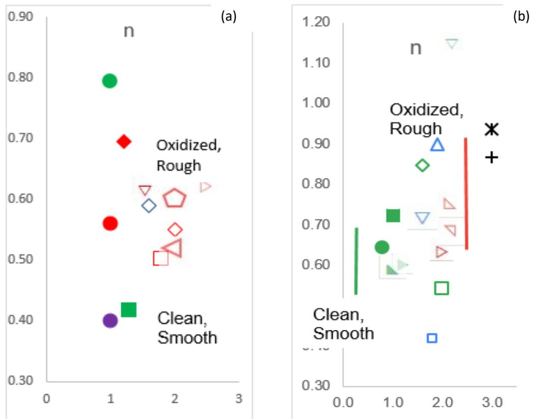
FIG. 4.9. Values of the high-energy SEY fitting parameter ( $n$ ) used in Eq. 2.2. Al studies (a) and Cu studies (b) listed in Tables 4.1, 4.3 are the source. The three columns of symbols in each plot displays values for smooth, rough, and unknown surface layers, respectively. Figure 4.2 identifies the plotting symbols used in these plots and listed for each specific study.
