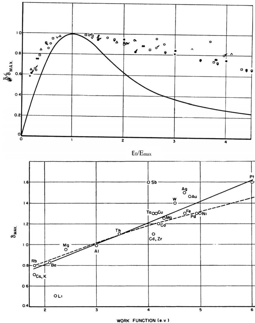
FIG. 2.8. Historical plots of reduced SEY. Plots as taken from Baroody (1950). Showing (a) reduced yield ( $\delta/\delta_{max}$ ) versus reduced Energy ( $E_0/E_{max}$ ) and (b) maximum yield ( $\delta_{max}$ ) versus work function ( $\Phi$ ).
