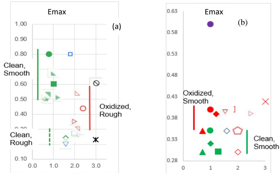
FIG. 4.2. Comparison of  $E_{max}$  values for various conducting samples. With (a) copper, and (b) aluminum. Included with aluminum is a measurement of  $Al_2O_3$  (Sapphire) to illustrate an extreme case of oxidation. Apparent from these graphs is the difference that an oxide layer has on  $E_{max}$  values. (Conductive oxides increase values, while insulating values decrease  $E_{max}$  values).
