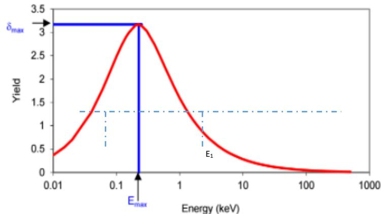
FIG. 2.6. Typical SEY yield curve with key features identified.
