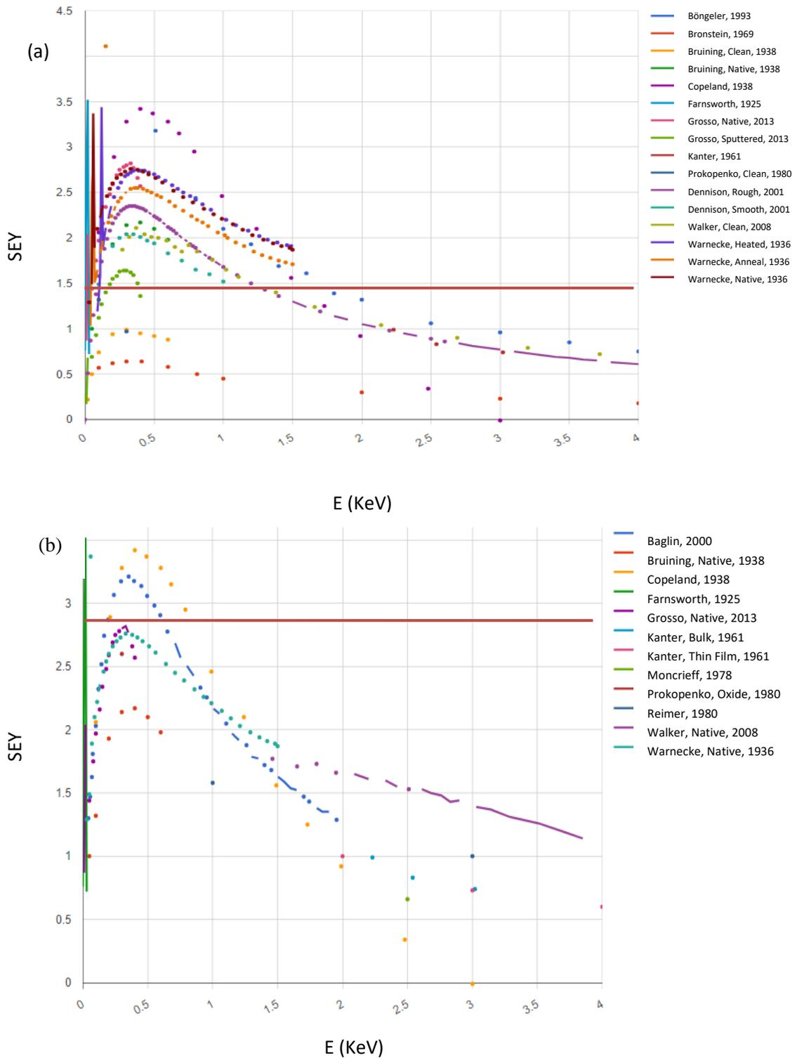
FIG. 3.11. Different aluminum SEY data sets sorted based upon surface contamination conditions. (a) clean, elemental and (b) contaminated and oxidized. Red lines are included to indicate average  $\delta_{max}$  values.
