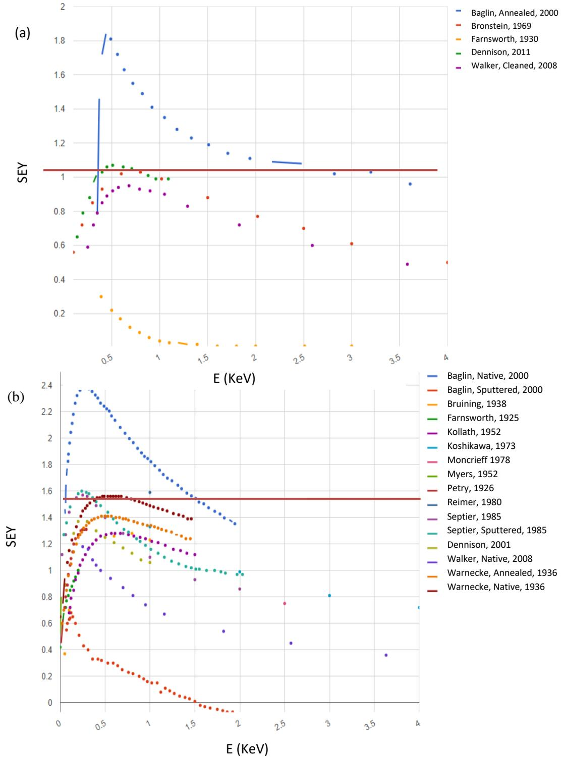
FIG. 3.10. Different copper SEY data sets sorted based upon surface morphology conditions. Figures show (a) smooth results and (b) rough results. Red lines are drawn in to indicate average  $\delta_{max}$  values.
