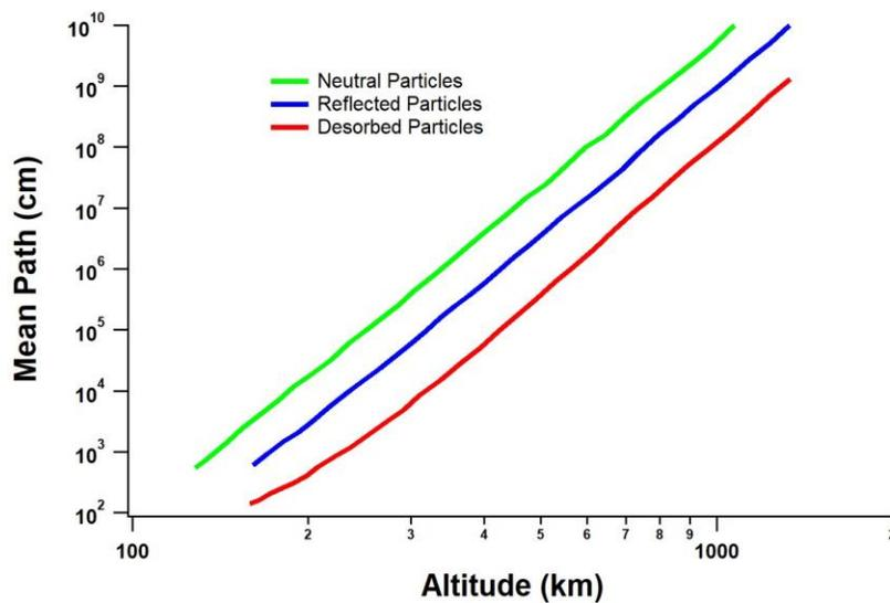
FIG. 4.7. Mean free paths versus altitude. The mean thermal velocity of the desorbed molecules is assumed to be  $v_D$  to be  $4 \times 10^4 \text{ cm s}^{-1}$ . The average velocity of the reflected particles is assumed to be one-third of the orbital velocity ( $v_R = v_0/3$ ) (Scialdone 1972).
