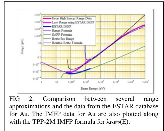
FIG 2. Comparison between several range approximations and the data from the ESTAR database for Au. The IMFP data for Au are also plotted along with the TPP-2M IMFP formula for  $\lambda_{IMFP}(E)$ .
