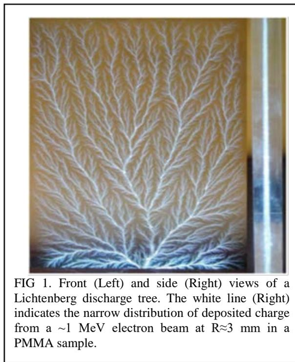
FIG 1. Front (Left) and side (Right) views of a Lichtenburg discharge tree. The white line (Right) indicates the narrow distribution of deposited charge from a ~1 MeV electron beam at  $R \approx 3$  mm in a PMMA sample.
