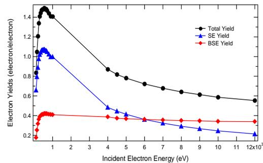
**Fig. 6** - Total SE and BSE yields as a function of incident electron energy for Cu.
