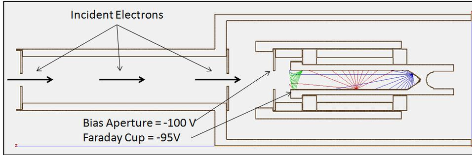
**Fig. 4** Theoretical SEs (green, red, and blue groups), each electron in each group has a  $KE=2$  eV. Each line represents the path line of an electron. The trajectory for each electron originates at the point source (where an incident PE might have impacted) and moves outward along its path line.
