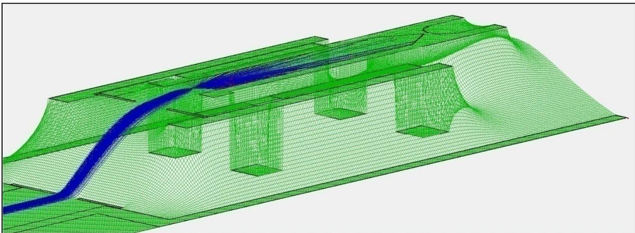
**Fig. B3** Electron capture visualization – electrons (blue) move from left to right. Potential energy contours (green) graphically show how much energy the incident electrons need to make it into the Faraday cup. Faraday cup = -100 V, Bias Aperture = -90 V, E-Beam = 100.1 eV
