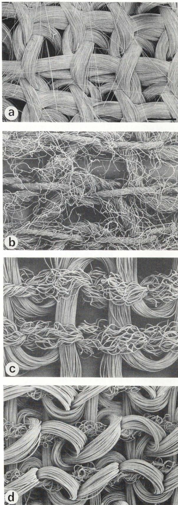
Figure 2 Scanning electron micrograph showing the knitted pattern of the following bandage fabrics: (a) Dynacast Extra (glass fibre) (b) Deltacast (cotton), (c) Deltacast Plus (polyester) and (d) Dynacast Pro (polypropylene and Lycra). Bar line (for all 4 figures) = 1mm.
