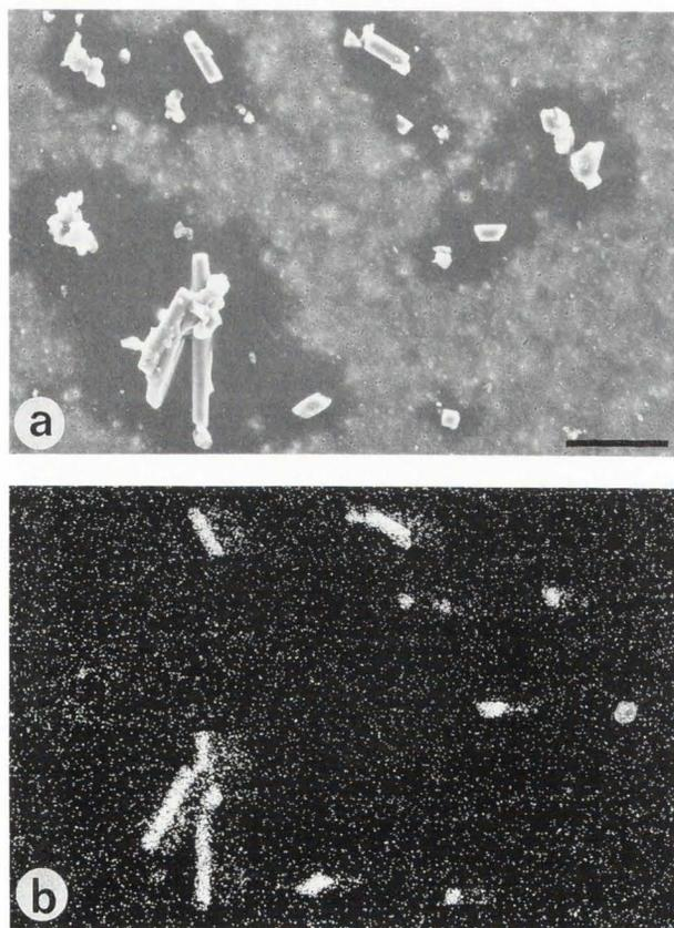
Figure 4 (a) Scanning electron micrographs showing a typical sample of dust collected during cutting of Dynacast Extra, a PU-impregnated glass fibre fabric bandage. (b) an X-ray dot map of the same area shown in (a) produced by the SiK and CaK X-rays generated from the glass component. Bar line (for both figures) = 50µm.
