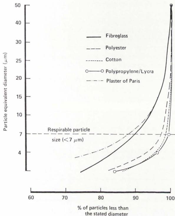
Figure 5 Particle size distribution of airborne dust generated during cutting of the plaster of Paris and synthetic bandages.
