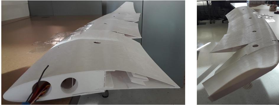
**Fig. 19** Discrete deflection on Horizon wing-segment (P18I17S04 - P18I17S07).
