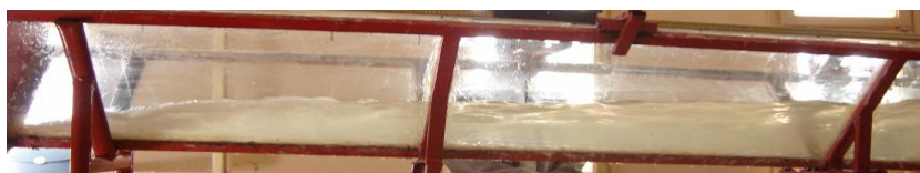
Figure 4. Hydraulic jump in a sloped triangular channel
