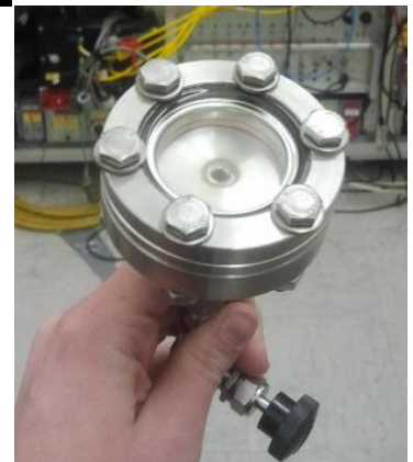
Figure 12, (bottom right) Mini vacuum chambers were assembled to house the samples during the UV
