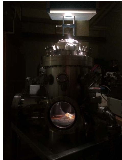
Figure 2: SST chamber with CubeSat setup.
