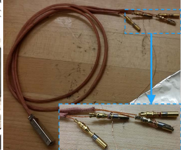
Figure 10: USB type B cable with an enlarged view of the sockets used for the cabling feedthrough.
