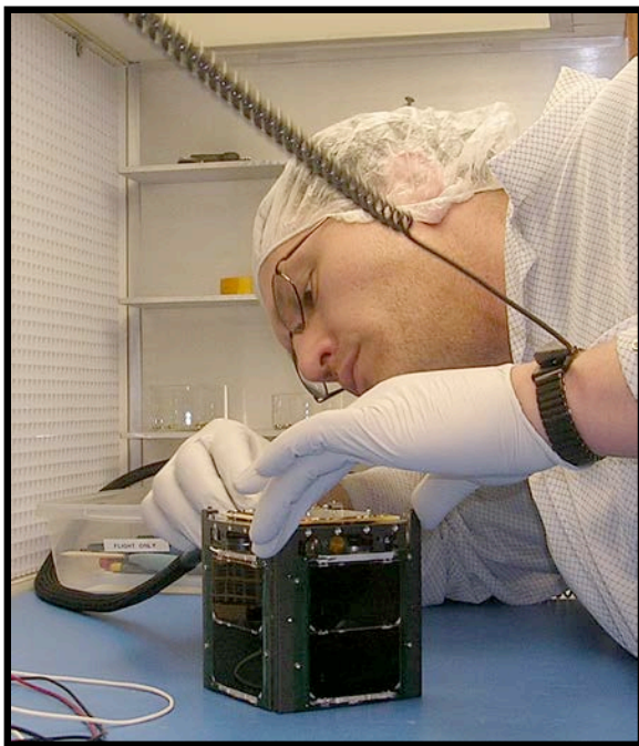
Figure 2: Keith Mashburn an MSU SSEL Physics graduate is shown putting final touches on the Explorer-1 [Prime] CubeSat.
