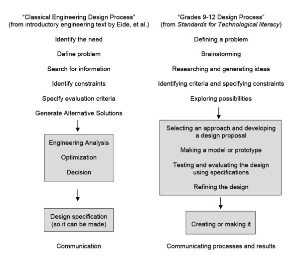
Comparison of an Introductory Engineering Design Process with the Standard 8 Design
