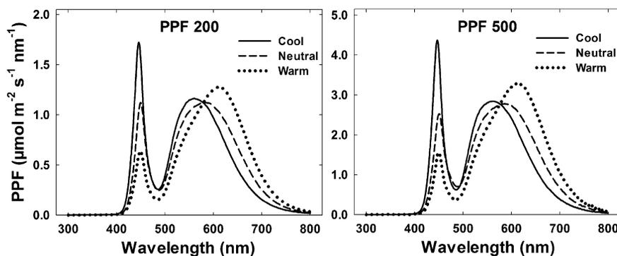
Fig. 2. Spectral distribution of warm, neutral, and cool white LEDs at 200 and 500  $\mu\text{mol}\cdot\text{m}^{-2}\cdot\text{s}^{-1}$ . Both spectra are shown because overdriving the LEDs to achieve 500  $\mu\text{mol}\cdot\text{m}^{-2}\cdot\text{s}^{-1}$  caused a slight spectral shift in all three LED types. LED = light-emitting diode.
