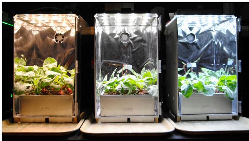
Fig. 1. Experimental set-up showing growth chambers, LED arrays, root modules, and thermocouples. The crop shown is radish on the day of harvest. Note the differences in plant form across treatments, which are arranged (left to right) warm, neutral, and cool white LEDs. LED = light-emitting diode.
