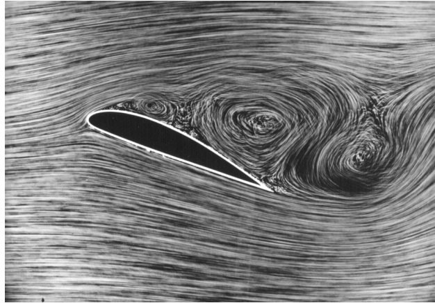
Fig. 1 Burble behind an airfoil; from [5].
