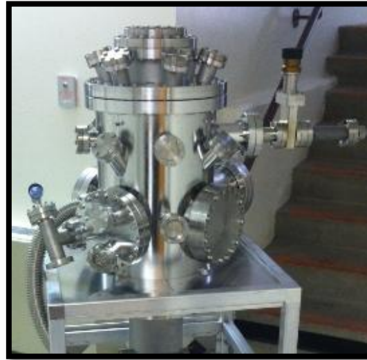
Figure 3 – The Space Survivability Test Chamber used to simulate the space environment in a controlled ground-based setting.
