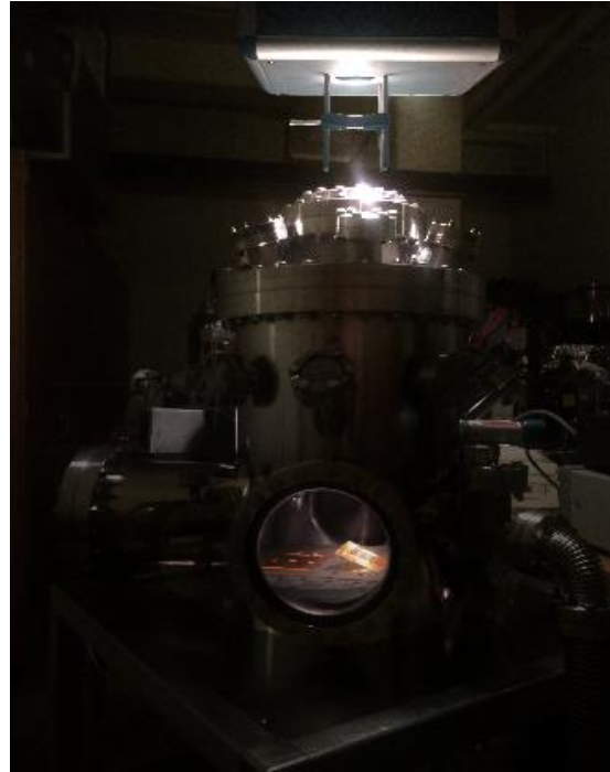
Figure 5 – SST Chamber with solar-cell degradation test setup. Sample carousel is visible through the chamber viewport.
