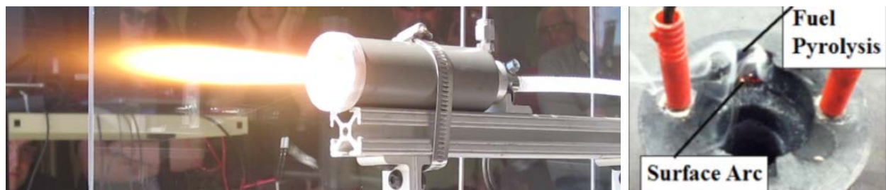
Figure 1. Test firing of thruster at Utah State University (left) and close up of 3D-printed fuel grain (right).
